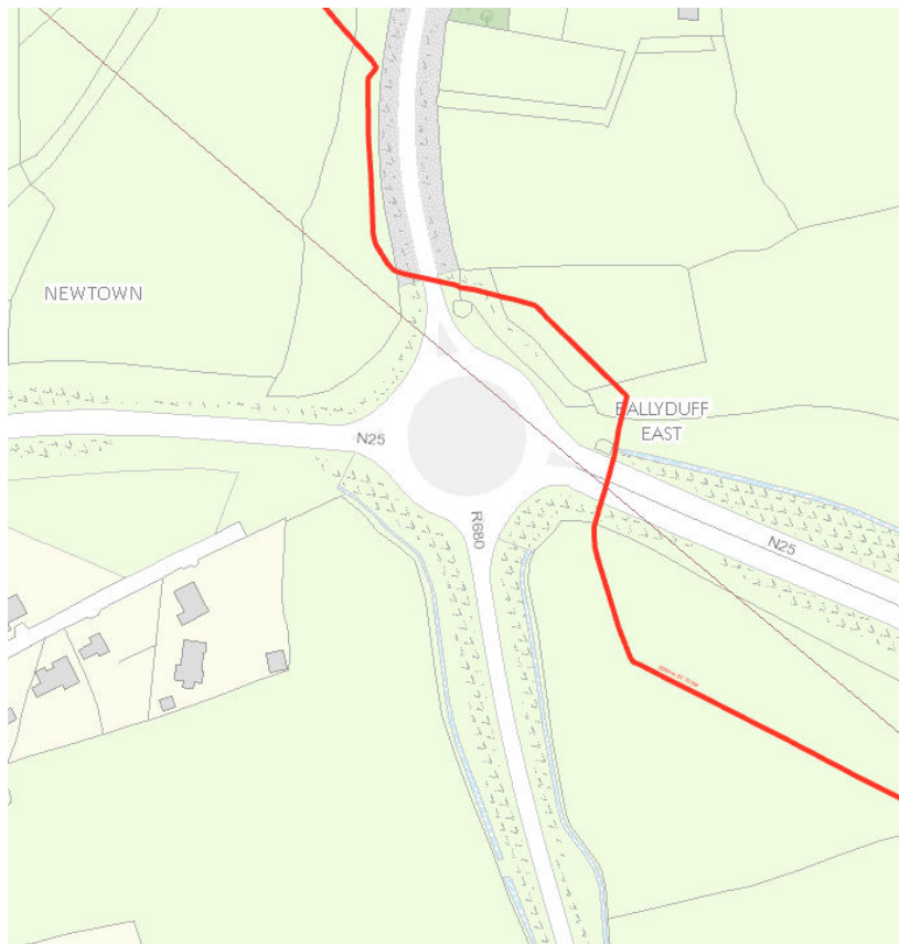
Figure 11.1 Gas mains line adjacent to Carrick Rd. Roundabout on the N25
